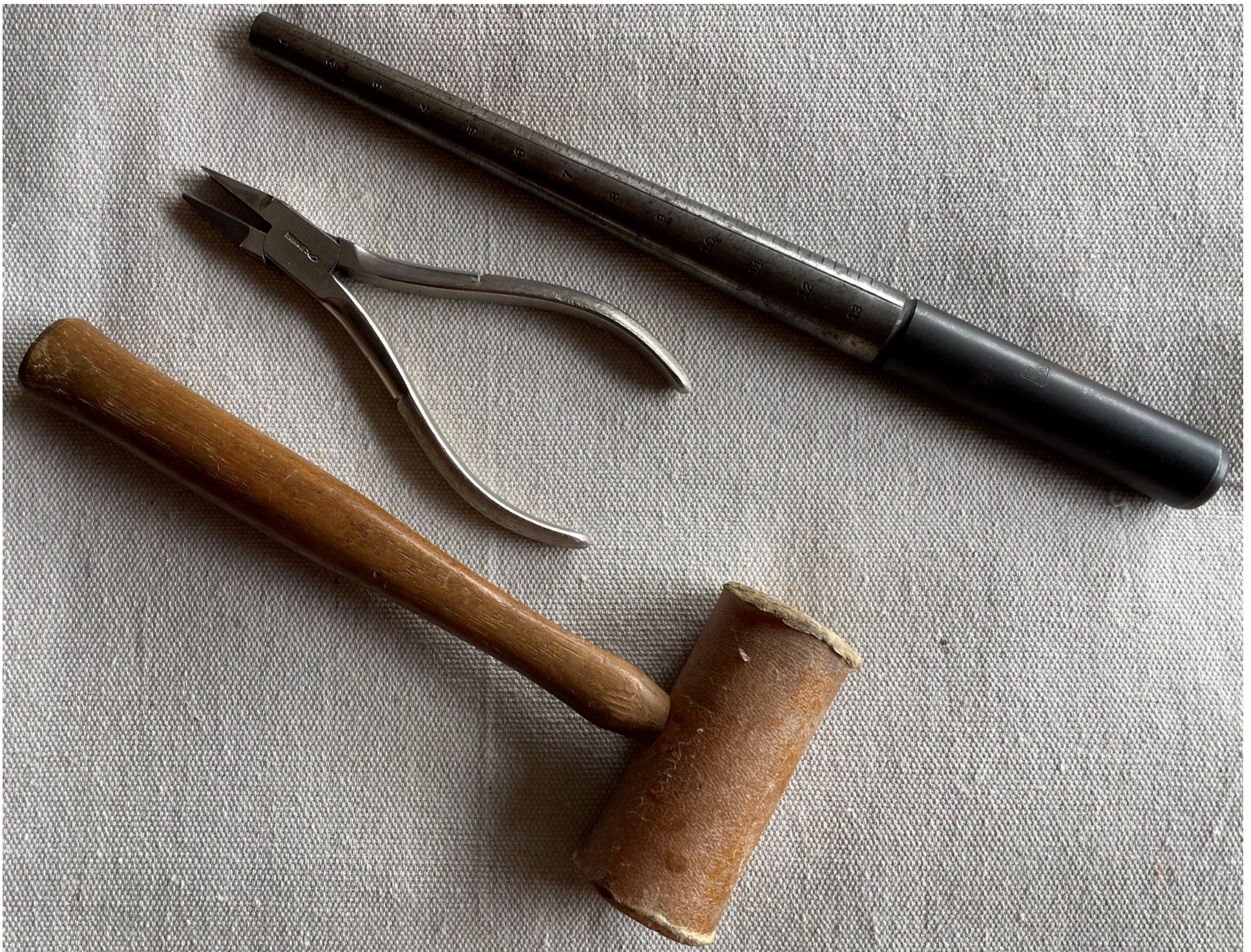
Jeweler's tools belonged to George L Buhler, now in possession of George L Buhler Jr. Steel ring mandrel, jeweler's flat nosed pliers and rawhide leather mallet.
